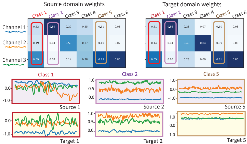
Figure 5.4: The top row shows channel weights learned by our model on the HHAR dataset for the corresponding input data below. The overall weight distribution across the two domains is mostly similar. The colored boxes highlight how weights learned for different classes help mask channels with larger shifts between the domains, contributing to improved domain adaptation performance.
